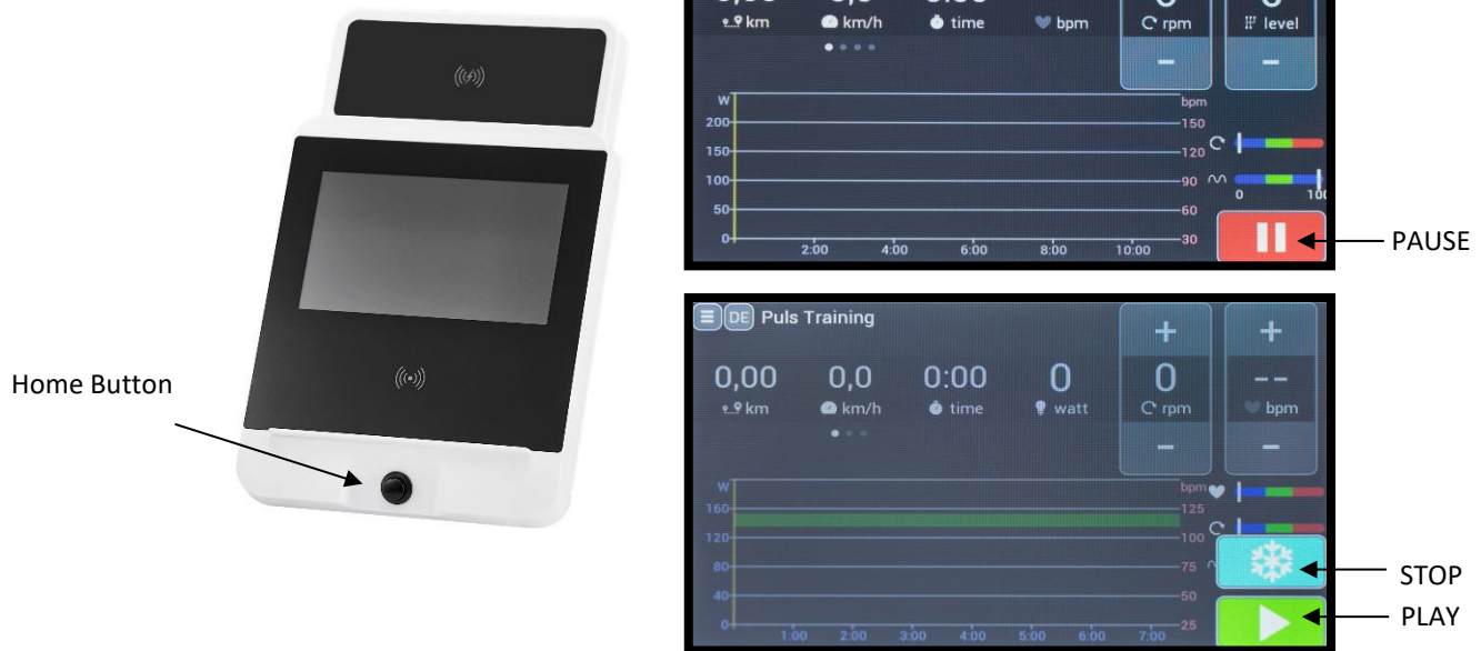
Fig. 2: Monitor view, explaining the button functions, actual view may vary in colour, button assignment is the same.
